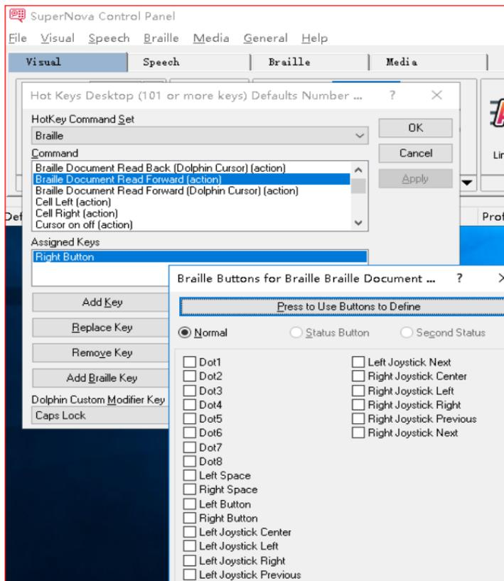
5. Press the Seika Braille notetaker button which you want to use and click "OK" button on the "Braille Buttons for Action" dialog. For example, you press dot8 in the Seika Braille notetaker, then the Dot8 will be marked in the below dialog automatically.
