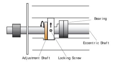
Loosen the locking screw, while lightly striking the adjusting stem, if you turn towards the direction of the arrow, the dots will be higher; in the opposite direction, they will be lower.
